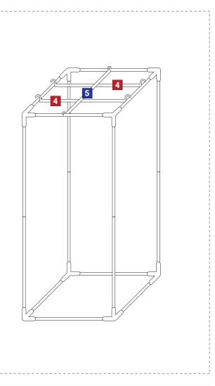
Fit the ceiling hanging bars inside the tent as shown. Insert (4) first and then place (5) on top. These poles can be moved arround to accomodate for different equipment.
