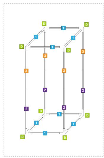
Assemble the frame by attaching the poles into the corner units (D) as shown above. Make sure that the poles are securely pressed into the corner unit, (you will hear a clicking sound).
