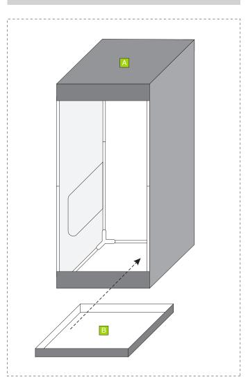
Carefully slip the canvas cover (A) onto the constructed frame and zip closed. Unzip the front door and place the floor tray (B) into the bottom of the tent.
