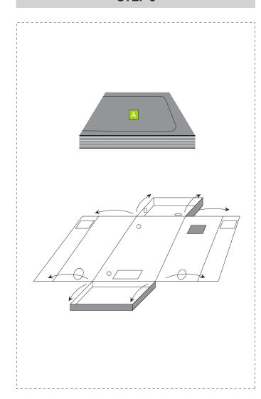
Lay out the grow tent canvas cover (A) on the floor. Place the tent frame on top of the canvas floor panel making sure that it is inserted the correct way.
