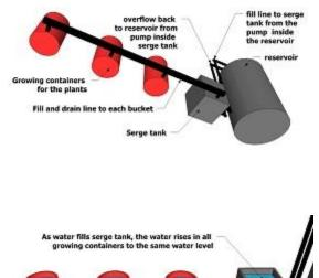
serge tank serves as a temporary reservoir that controls the water height in all the containers with the plants in them, and is only full during the flooding cycle.
