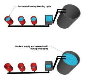
After the timer for the pump in the main reservoir shuts off, the pump in the serge tank is still on. The pump in the serge tank continues pumping all the water back into the main reservoir (draining the system) until the water level gets low enough. At that point a second float valve shuts off the pump in the serge tank.
